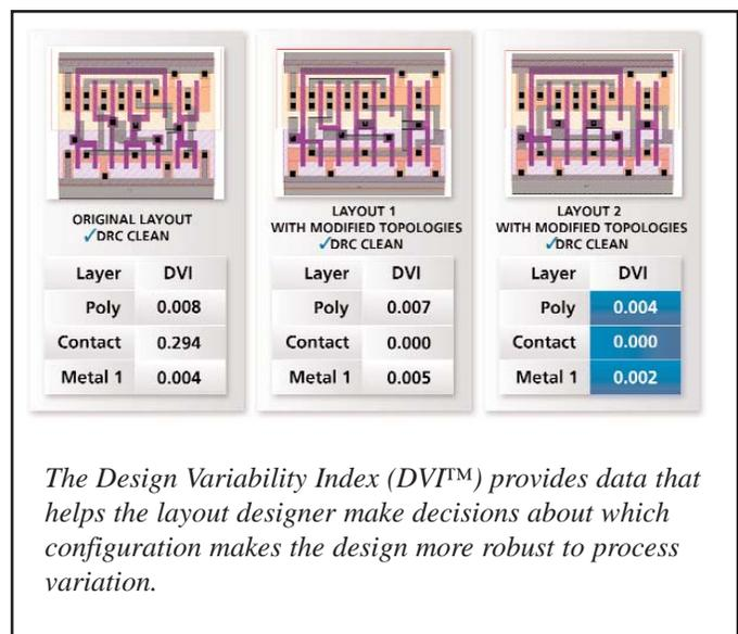
The Design Variability Index (DVI™) provides data that helps the layout designer make decisions about which configuration makes the design more robust to process variation.
