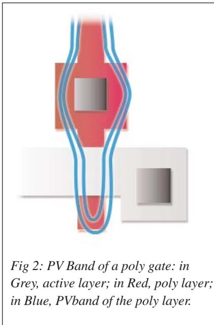
Fig 2: PV Band of a poly gate: in Grey, active layer; in Red, poly layer; in Blue, PVband of the poly layer.
