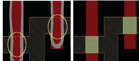
Calibre LFD uses process variation (PV) bands that predict failure in common configurations including pinching, bridging, area overlap and CD variability.
