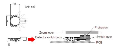
Fig. 1: The lever of the switch is long and higher above the PCB than the switch body, making it easier for the protrusion on the zoom lever to catch.
